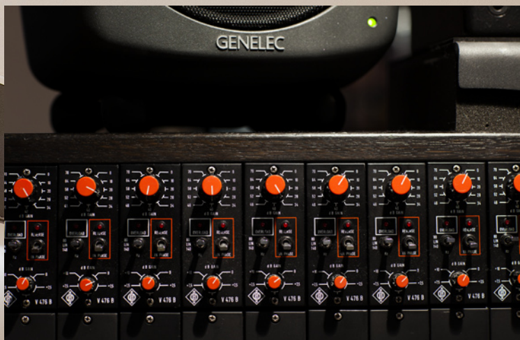
Clockwise from top left: the Neumann console from 1990 is equipped with 32 V476b preamp modules; unusual outboard units include an Orban parametric EQ, a Spectra Sonics 610 Compliter and a BAE 10x2 mixer; classic compressors on offer include a Chandler TG1, Retro Instruments Sta-L level and Universal Audio 1176LN; and vintage AKG C24 and Neumann U47 and U67 valve mics.
