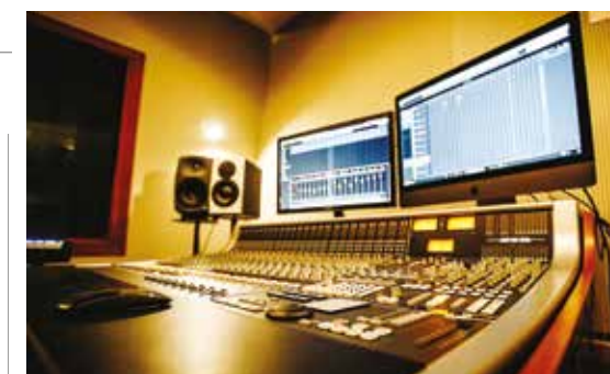
The SSL AWS 924 conected to an iMac running Avid Pro Tools
